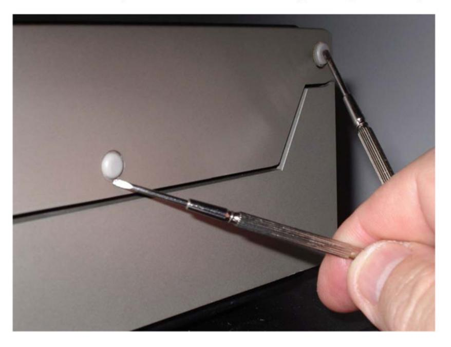
The rivets are made of 2 or 3 pieces. You must disassemble 1 piece (of the 2 or 3 that forms the rivet) at a time. (also to assembly the rivets at the end of the job you must do it one piece at a time)
