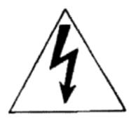
This symbol is intended to alert the user to the presence of uninsulated "dangerous voltage" within the product's enclosure that may be of sufficient magnitude to constitute a risk of electric shock to persons.
