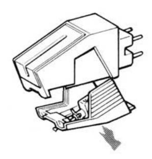
3 Plug the cartridge into the tonearm and tighten the cartridge locking screw firmly.
