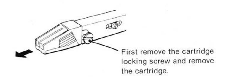
2 Detach the stylus assembly and insert a new stylus into the cartridge.
