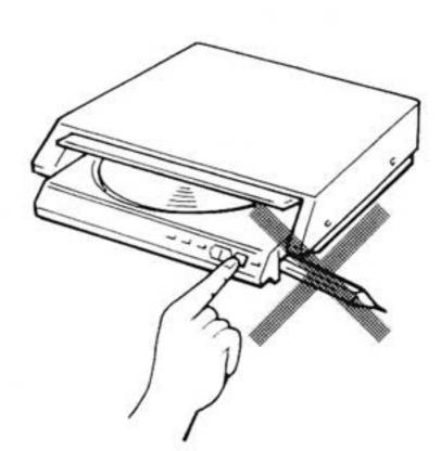
If the foreign object should be caught in this position, press the OPEN/CLOSE button immediately so that the module will move in the opposite direction.
