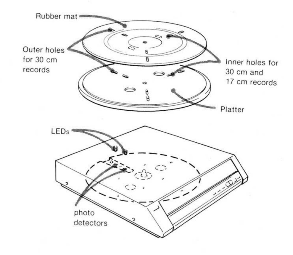
When a 30 cm record is to be played, both inner and outer holes are covered so no beam is transmitted to the photo detectors.
