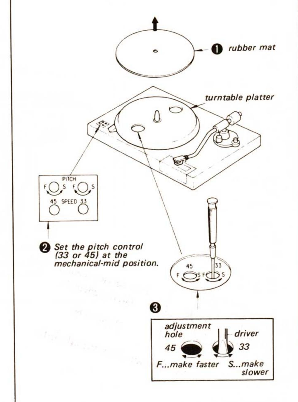
After the adjustment, touch the START/STOP button and confirm that the pattern appears stationary.
