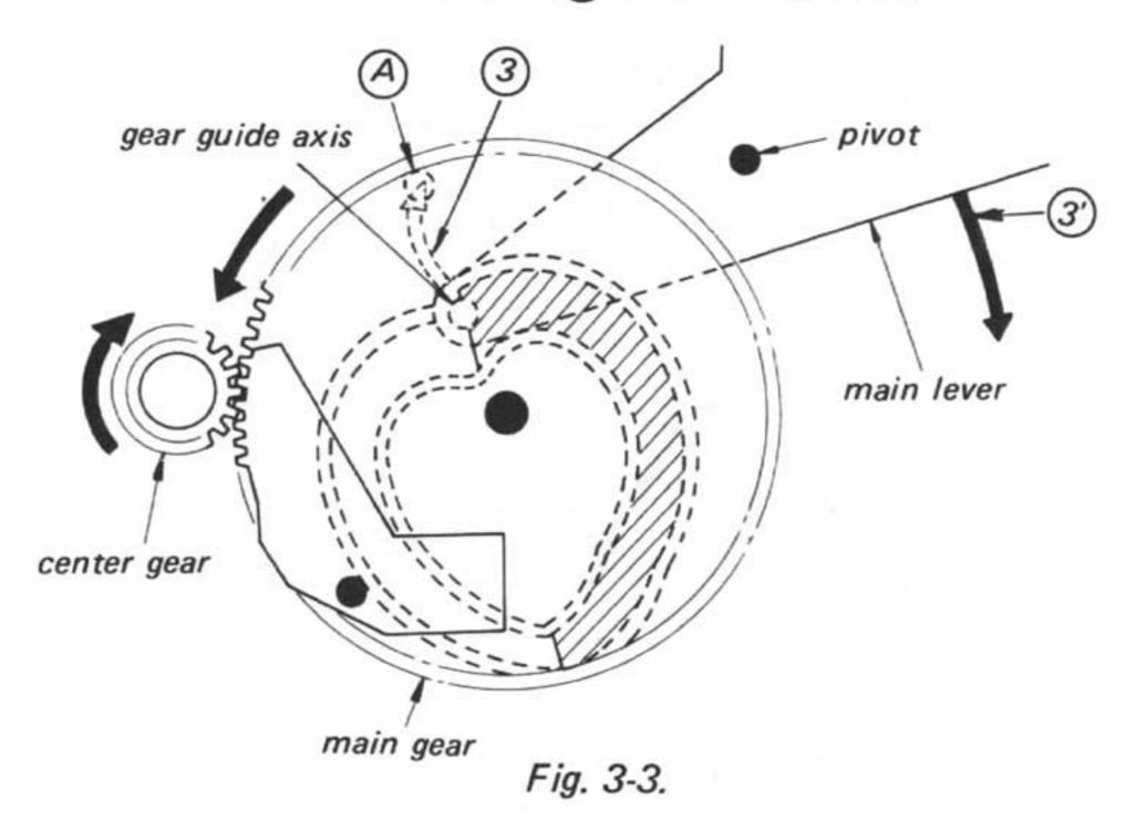
5. At this time, the lead-in lever moves in the direction of arrow 4, guided by the lead-in cam which moves together with the main lever. The tip D of the lead-in lever moves to position B, pushing against a pin on the brake drum in the direction of arrow 6. And since this brake drum moves in unison with the tonearm, the tonearm will moves across (horizontal movement) in the direction of arrow 5. (See Fig. 3-4.)
