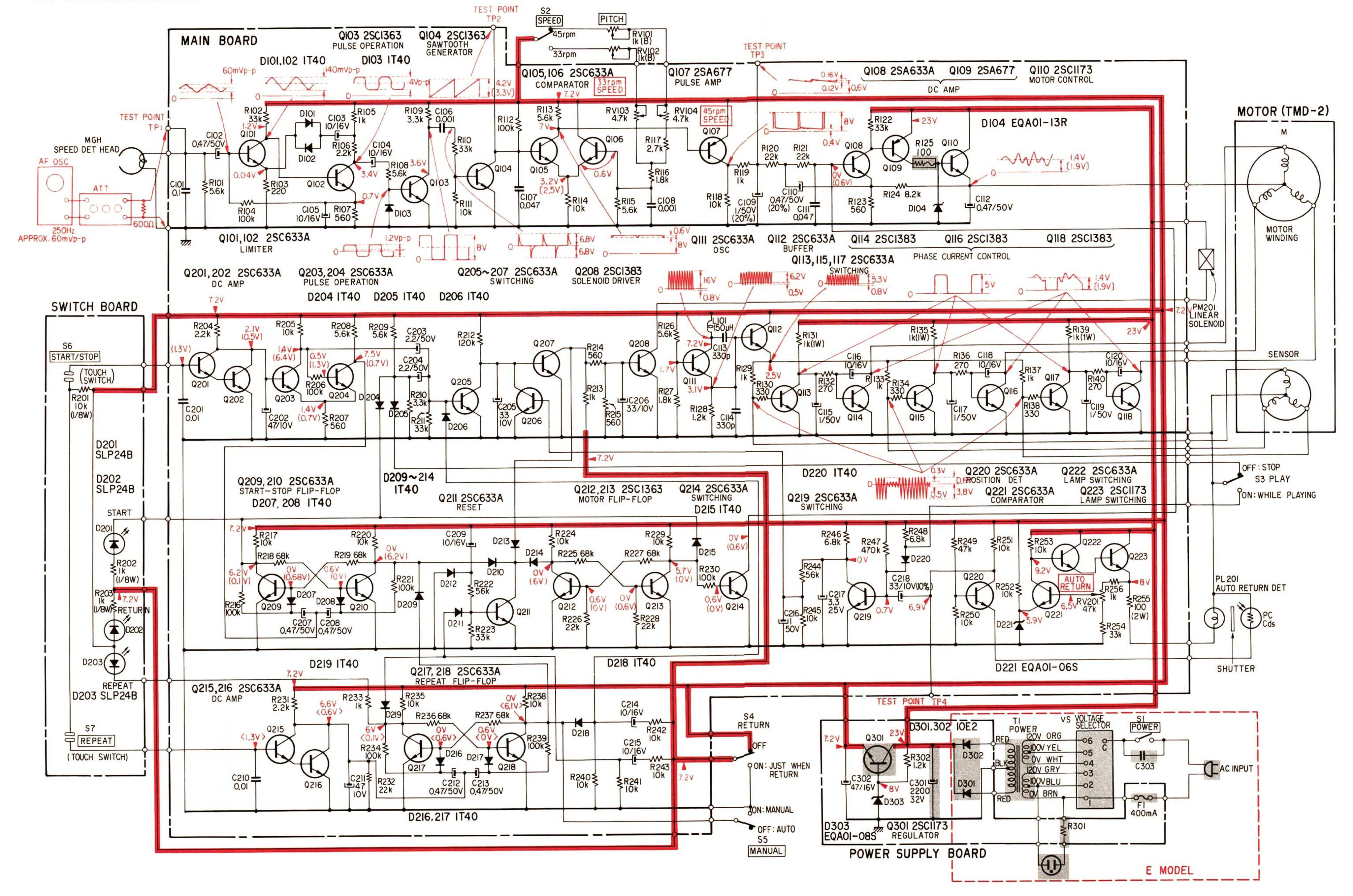
Note: The components identified by shading are critical for safety. Replace only with part number specified.
