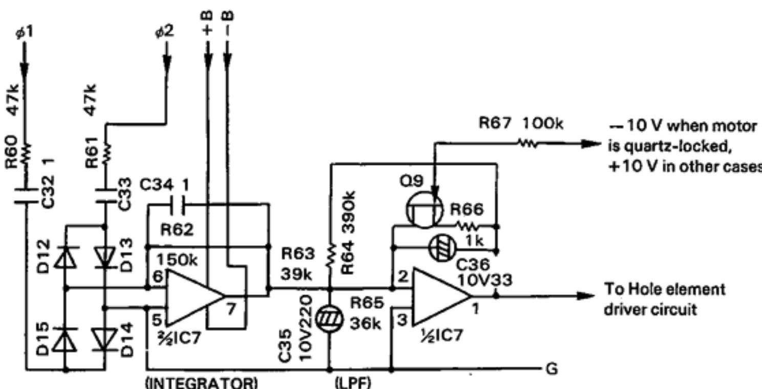
The positive side of  $\phi_1$  and negative side of  $\phi_2$  are input to the integrator, and the difference between  $\phi_1$  and  $\phi_2$  is output from it. (The difference between the ① and ② portions in the diagram on the left)
